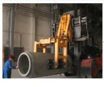
Grippers for concrete pipes:
