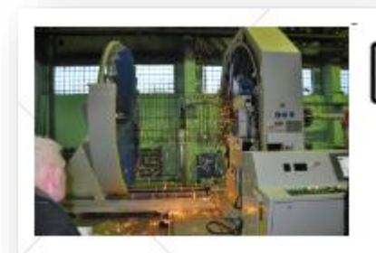
Welding cage machine for producing cages for pipes and manhole rings; producer mbk Maschinenbau GmbH (Germany), type BSM 450 - 33-300/24 LD 3000, construction year 2009,
