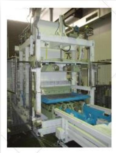
Concrete – block machine (vibropress) SP-2000
