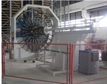
Welding cage machine for producing cages for pipes and manhole rings; producer mbk Maschinenbau GmbH (Germany), type BSM 450 - 33-300/24 LD 3000, construction year 2008
