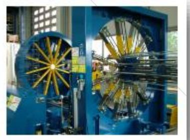
Welding cage machine for producing cages for pipes and
